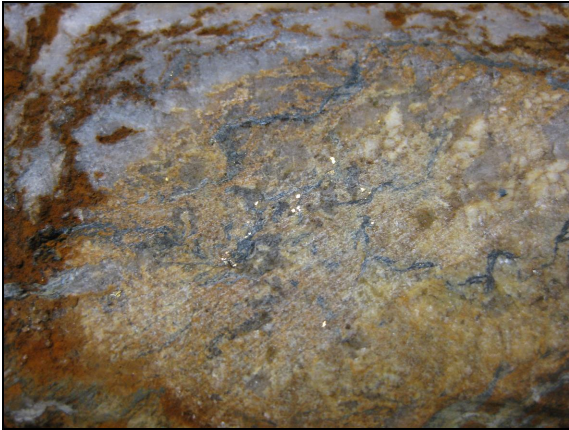
Photos illustrating the visible gold and associated alteration from Flint Mine stockpiles
