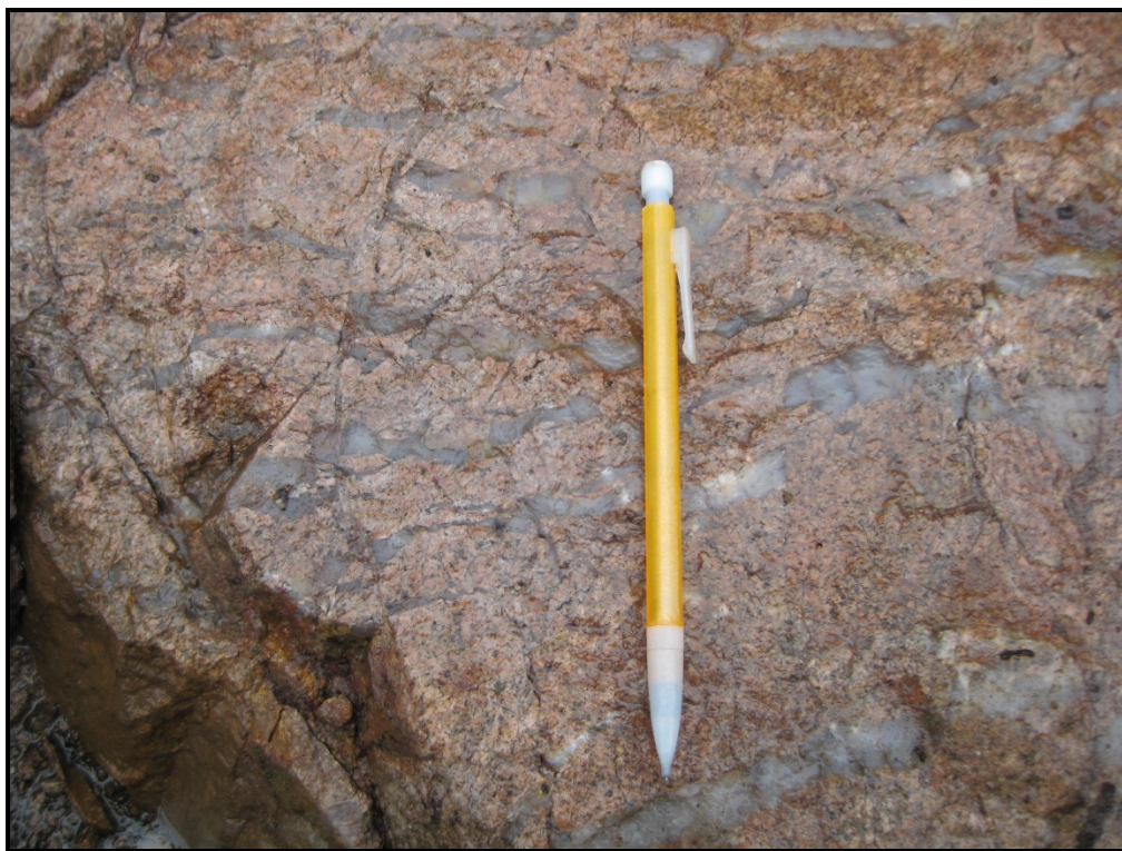
East-west oriented quartz veinlets cut and displaced by north-south structures (pencil pointing north)
