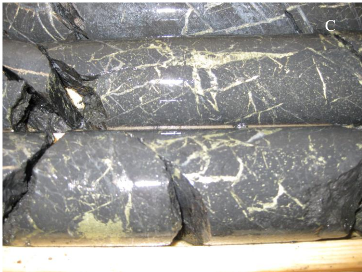
Plate A: Semi-massive to massive chalcopyrite in argillites Plate B: Nodule style chalcopyrite in argillites Plate C: Random/cross-cutting chalcopyrite stringers/veinlets Plate D: disseminated to stringer chalcopyrite conforming to bedding
